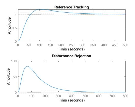
By default, for a given bandwidth, pidtune tunes the controller to achieve a balance between reference tracking and disturbance rejection. In this case, the controller yields some overshoot in the reference-tracking response. The controller also suppresses the input disturbance with a somewhat longer settling time than the reference tracking, after an initial peak.
