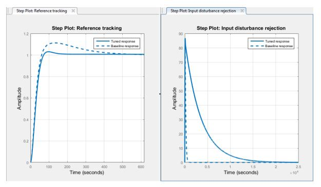
The PIDF controller tuned with reference-tracking focus is displayed as **Tuned response** (solid line). The plots show that the resulting controller tracks the reference input with considerably less
