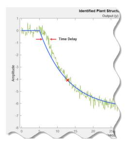
To add a transport delay to the estimated plant model, in the **Plant Structure** section, check **Delay**. A vertical line appears on the plot, indicating the current value of the delay. Drag the line left or right to change the delay, and make further adjustments to the system response by dragging the red x.
