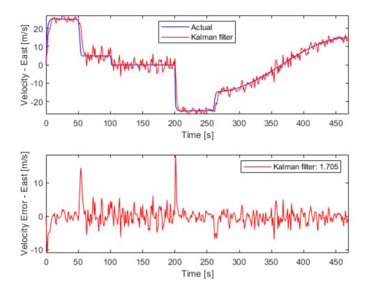
The legend on the error plot shows the east velocity estimation error  $||\dot{x}_e - \dot{x}_e||_1$  normalized by the number of data points.
