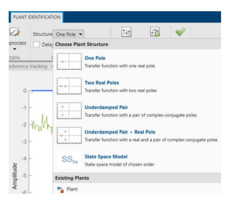
For any chosen structure you can optionally add a delay, a zero and/or an integrator element using the corresponding checkboxes. Click **Edit Parameters** to view the model transfer function configured by these choices.
