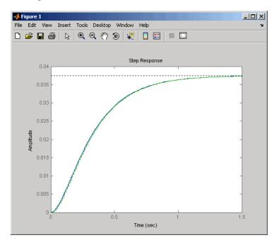
Note the step response match. Continuous and FOH-discretized step responses match for models without internal delays.
