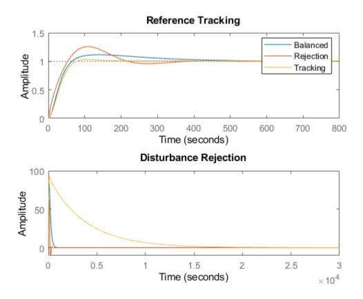
When you use the DesignFocus option to favor reference tracking or disturbance rejection in the tuned control system, you can still adjust phase margin for further fine tuning of the balance between these two measures of performance. Use DesignFocus and PhaseMargin together to achieve the performance balance that best meets your design requirements.
