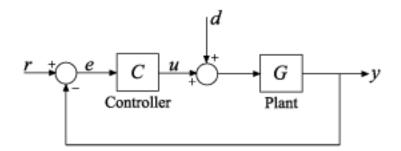
Setpoint tracking is the response at y to signals at r. Input disturbance rejection is the suppression at y of signals at d.
