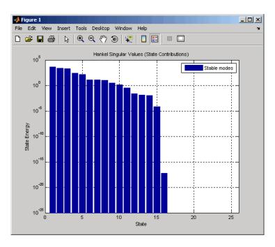
Small Hankel singular values indicate that the associated states contribute little to the I/O behavior. This plot shows that discarding the last 10 states (associated with the 10 smallest Hankel singular values) has little impact on the approximation error.
