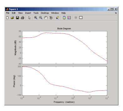
As the overlap of the curves in the figure shows, the reduced model provides a good approximation of the original system.
