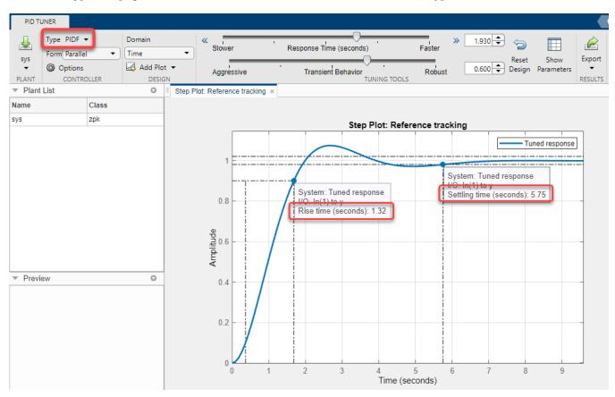
In the **Type** menu, select **PIDF**. **PID Tuner** designs a new PIDF controller. (See "PID Controller Type" on page 4-5 for more information about available controller types.)
