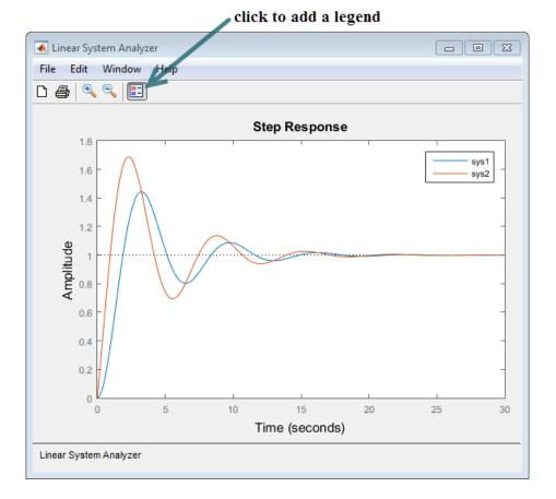
**Note** Alternatively, open Linear System Analyzer from the **Apps** tab in the MATLAB desktop. When you do so, select **File** > **Import** to load linear models from the MATLAB workspace or a MAT file.
