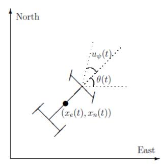
$x_e(t)$  and  $x_n(t)$  are the vehicle's east and north positions from the origin,  $\theta(t)$  is the vehicle orientation from east and  $u_{\psi}(t)$  is the steering angle of the vehicle. t is the continuous-time variable.
