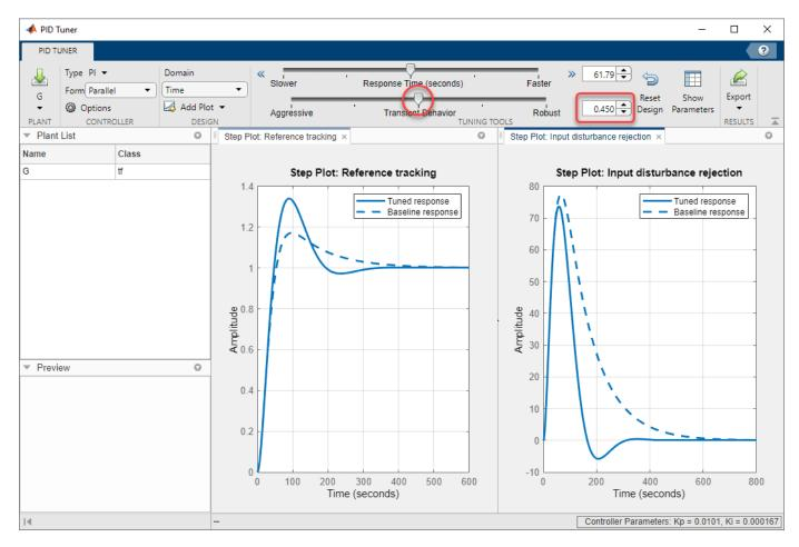
Lowering the transient-behavior coefficient to 0.45 speeds up disturbance rejection, but also increases overshoot in the reference-tracking response.
