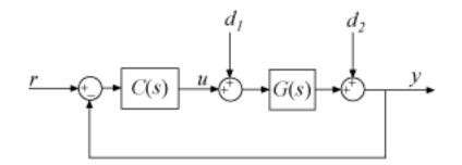
For 2-DOF PID controller types such as PI2, PIDF2, and I-PD, the software computes responses based upon the following architecture:
